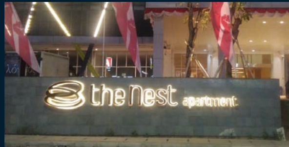
Client: Serpong Garden Apartement Location: Cisauk, Tangerang | Year: 2018 Material: Galvanized Steel, LED Lamp, Acrylic, Flexy German | Service: Building ID
